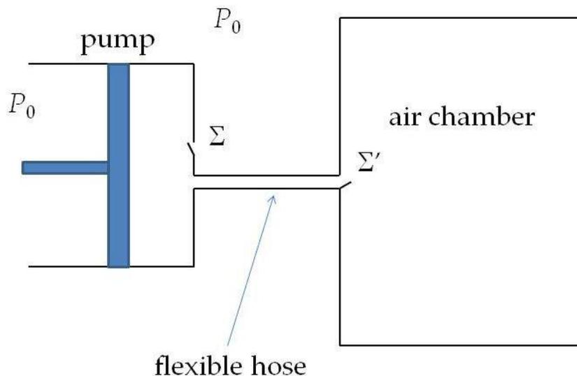
*Figure 1: Air chamber connected to a pump.*
